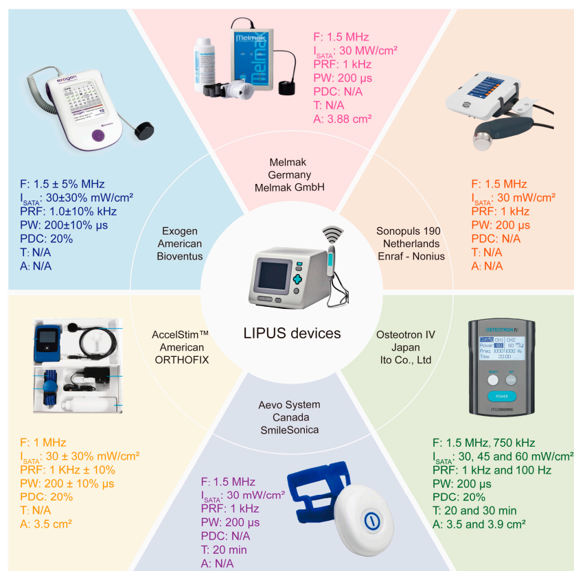
Figure 3. LIPUS devices and their parameters for experimental research and clinical use in different countries. Six LIPUS devices from five countries worldwide are listed, including the device names, the companies they belong to, and their countries of origin. Moreover, the different parameters that each device can modulate are listed in detail. LIPUS, low-intensity pulsed ultrasound; F, frequency; I_{SATA} , space-averaged time-averaged intensity; PRF, pulse repetition frequency; PW, pulse width; PDC, pulse duty cycle; T, exposure time; A, area of ultrasonic transducer; N/A, not available or not applicable.
